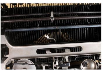
Step 2: Remove the tensioning spring
