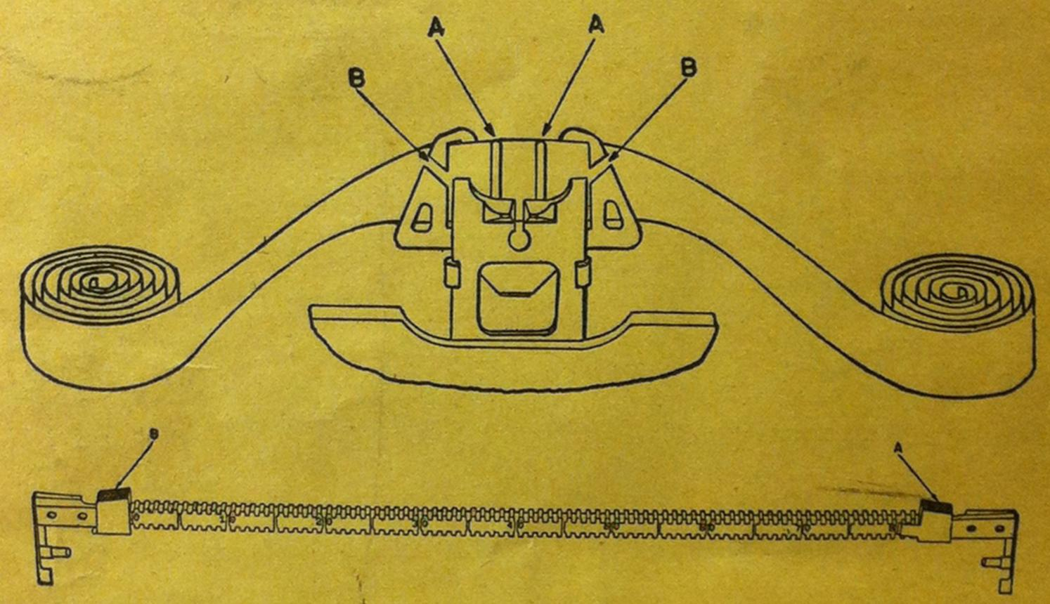
MARGINAL STOPS. Shown above govern the length of the writing line. They are easily reached by tilting the Paper Table backward and are moved by pressing against the corrugated sides. The Right Hand Stop (A) as you face the machine, governs the margin at end of line and rings bell. The Left Hand Stop (B) governs the margin at the beginning of line.
