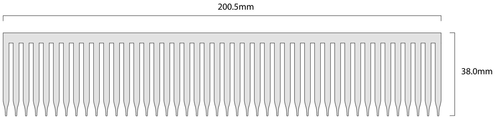
NOTE: material is .005' in thick tin-plated copper
