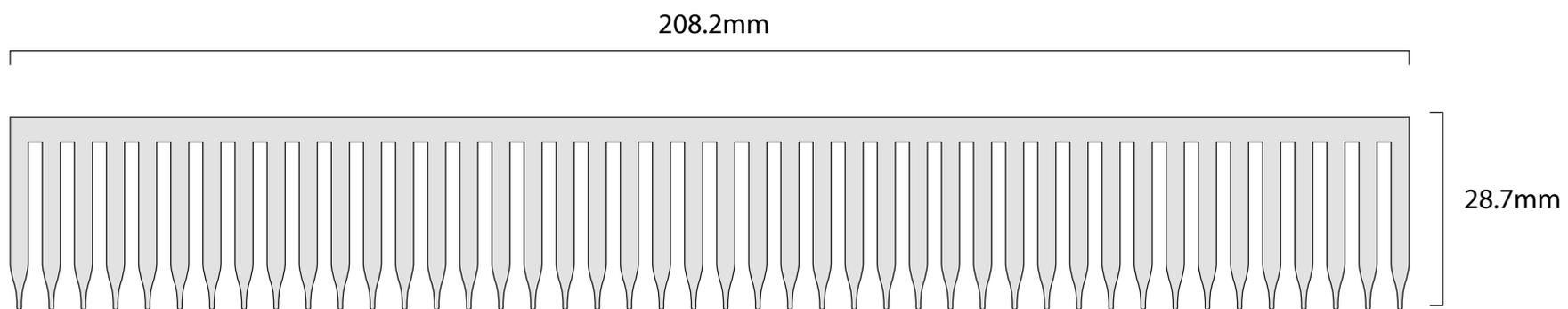
NOTE: material is .005 in thick tin-plated copper
